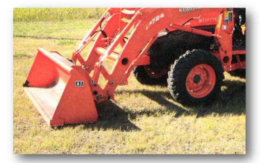
Heavy duty general purpose bucket can be used for almost any application. Use it for snow, grain, manure, light material, etc.
