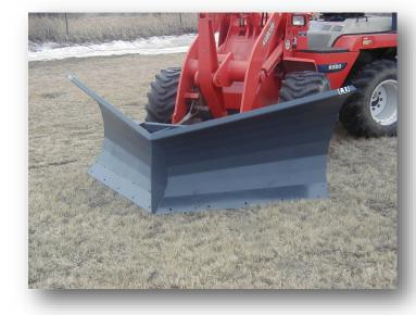
Fast and efficient way to remove snow from sidewalks and paths. Unloads snow equally right and left.
