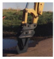
**Asphalt Cutter Backhoe Quick Couple Mount**
